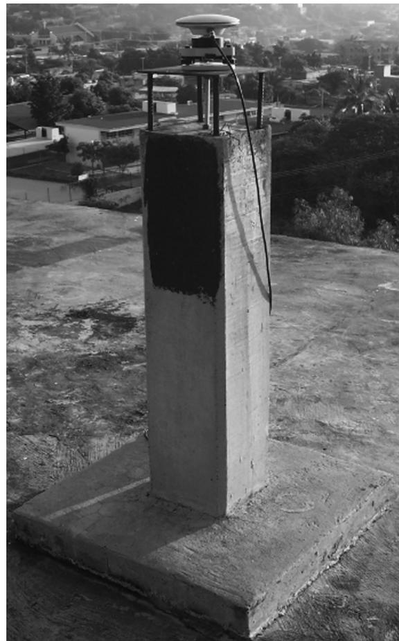
**Figure 3.** Monumentation of BASE 2 site, located on top of a facility building; UAS campus. GPS Receiver Leica SR500 with Leica (LEIAT502) antenna, collecting data on October 10, 2010.
