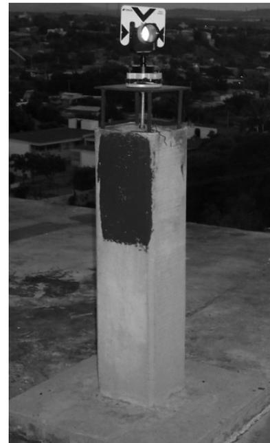
**Figure 7.** Prism location at BASE2 site, Topcon prism as an example.
