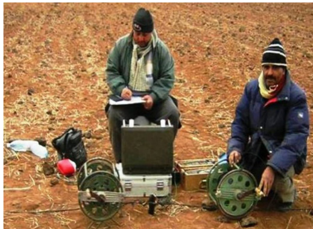
Figure 3 (a). VES Schlumberger configuration and its field operation in the field (Othman et al. , 2022).
