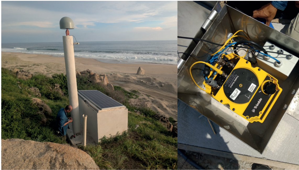
Figure 4. Seismogeodetic station Playa Banco de Oro (PYBO) in the state of Oaxaca (Figure 1). On the vault cover is the solar panel that independently feeds the station. On top of the concrete column the GNSS antenna is protected by a radome and on the side of the column is the UNI 3500 L-Band internet terminal (left). The radome , short for radar dome, is a protective enclosure that protects the GNSS antenna while allowing electromagnetic signals (radio, GNSS, radar) to pass through with minimal distortion. The concrete vault hosts the Kestrel seismogeodetic instruments, the ethernet switch, the batteries, and the solar charge controller (right).
